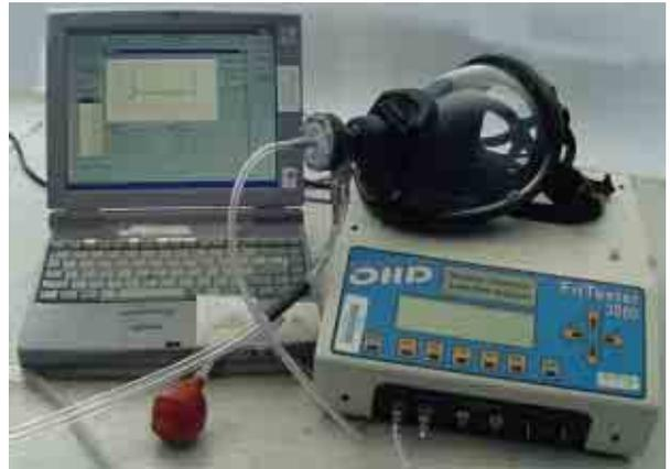
**Fig. 10 Controlled negative pressure fit testing device**
